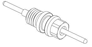
All PEEK, Reinforced PEEK or Glass-to-Metal-Sealed.
